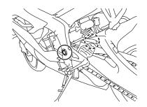
The swingarm pivots must be lubricated by a Yamaha dealer at the intervals specified in the periodic maintenance and lubrication chart.
