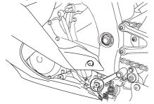
The operation of the brake and shift pedals should be checked before each ride, and the pedal pivots should be lubricated if necessary.
