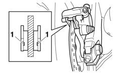
1. Brake pad wear indicator groove
