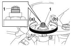
1. Spring preload adjusting bolt
