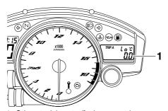
Odometer/tripmeter/fuel reserve tripmeter/stopwatch
