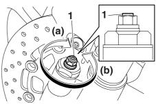
Compression damping force adjusting bolt (for slow compression damping)
